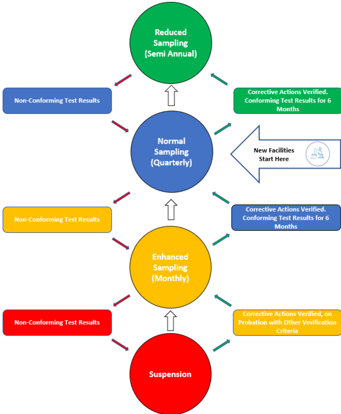
Finished Product Sampling and Testing flow chart (described in Annex 4 Table I).
